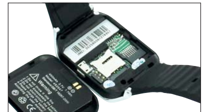
Its own SIM-Card makes SWP33X an independent Mobile Phone
